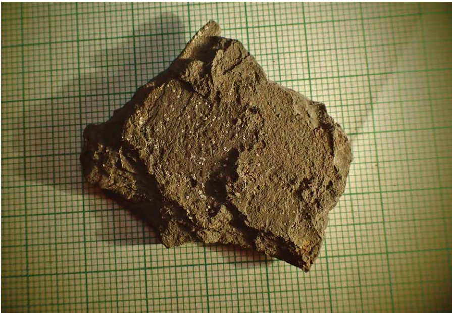
Figure 16. Gypsum inclusions on shale surface, 1 mm background grid.
