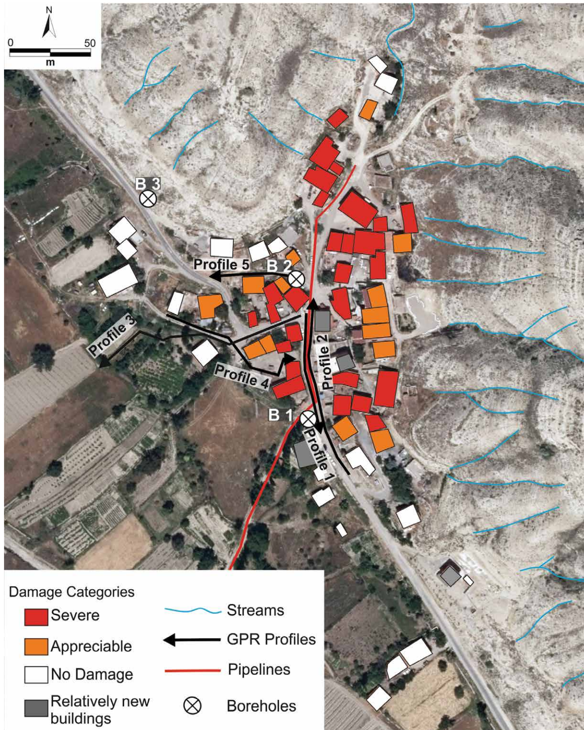
Figure 5. Map of damage distribution in March 2017 showing location of boreholes, GPR profiles (Özçelik et al. 2016) and pipeline.
