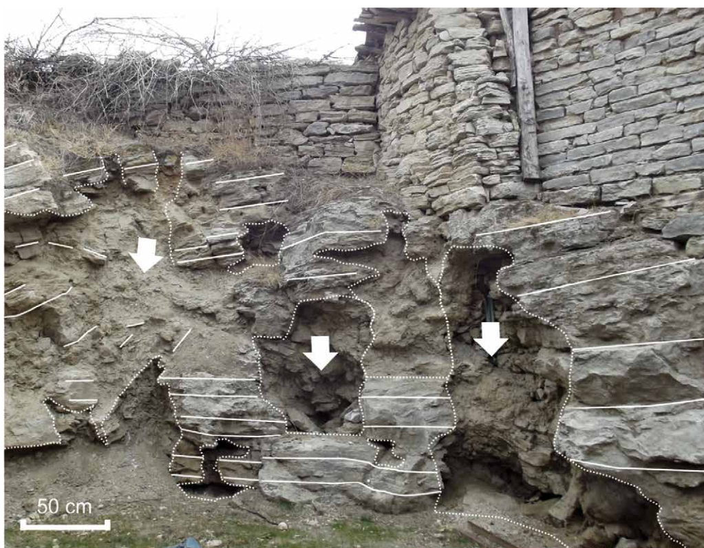
Figure 3. Paleo-subsidence structures in gypsum bedrock. Cavities are filled with karstic residue and gypsum blocks. (Photograph taken on eastern slope of village).
