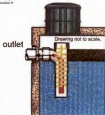
Figure 2: Diagram of installed filter and Tee Baffle. Note: drawing is not to scale.
