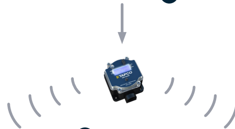
2 Activated BLINKERBEAM® TRANSMITTER RADIO sends wireless signal to receiver(s)
