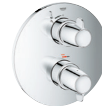
29 094 000 + 35 500 000 Grotherm Special Thermostatic shower mixer with safety stop between 35 °C and 43 °C + GROHE Rapido T thermostatic mixer for concealed installatio
