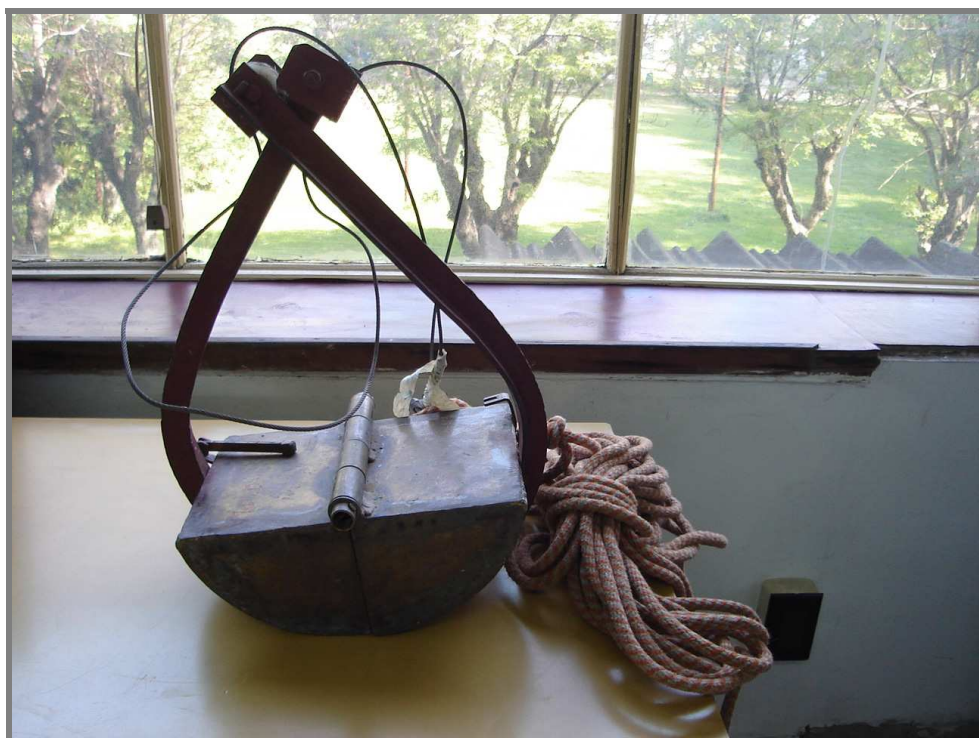
Fig. 2. Van Veen dredge used for collecting the benthic samples in Lower Uruguay River, Argentina.
