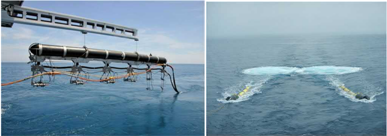
FIGURE 6-4: EXAMPLE OF A SEISMIC SOURCE (AIRGUN ARRAY) Source: TEPNA
