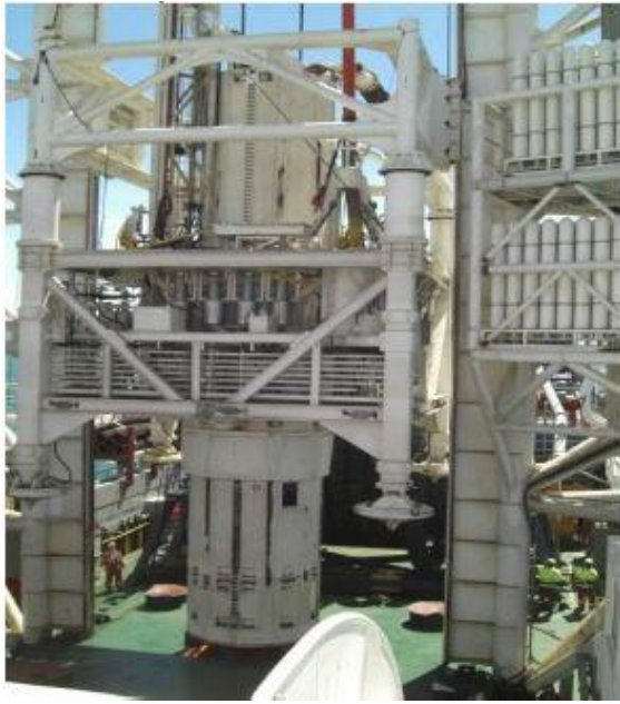
Figure 2: Illustrative example of a drill bit operated from a drill frame structure located onboard a vessel of opportunity.
