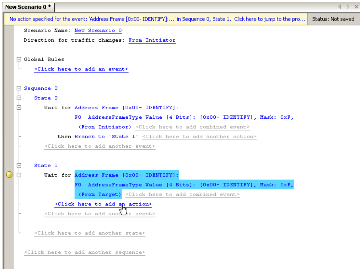
Figure 4.42: Example 7: Adding an Action to the Second State
