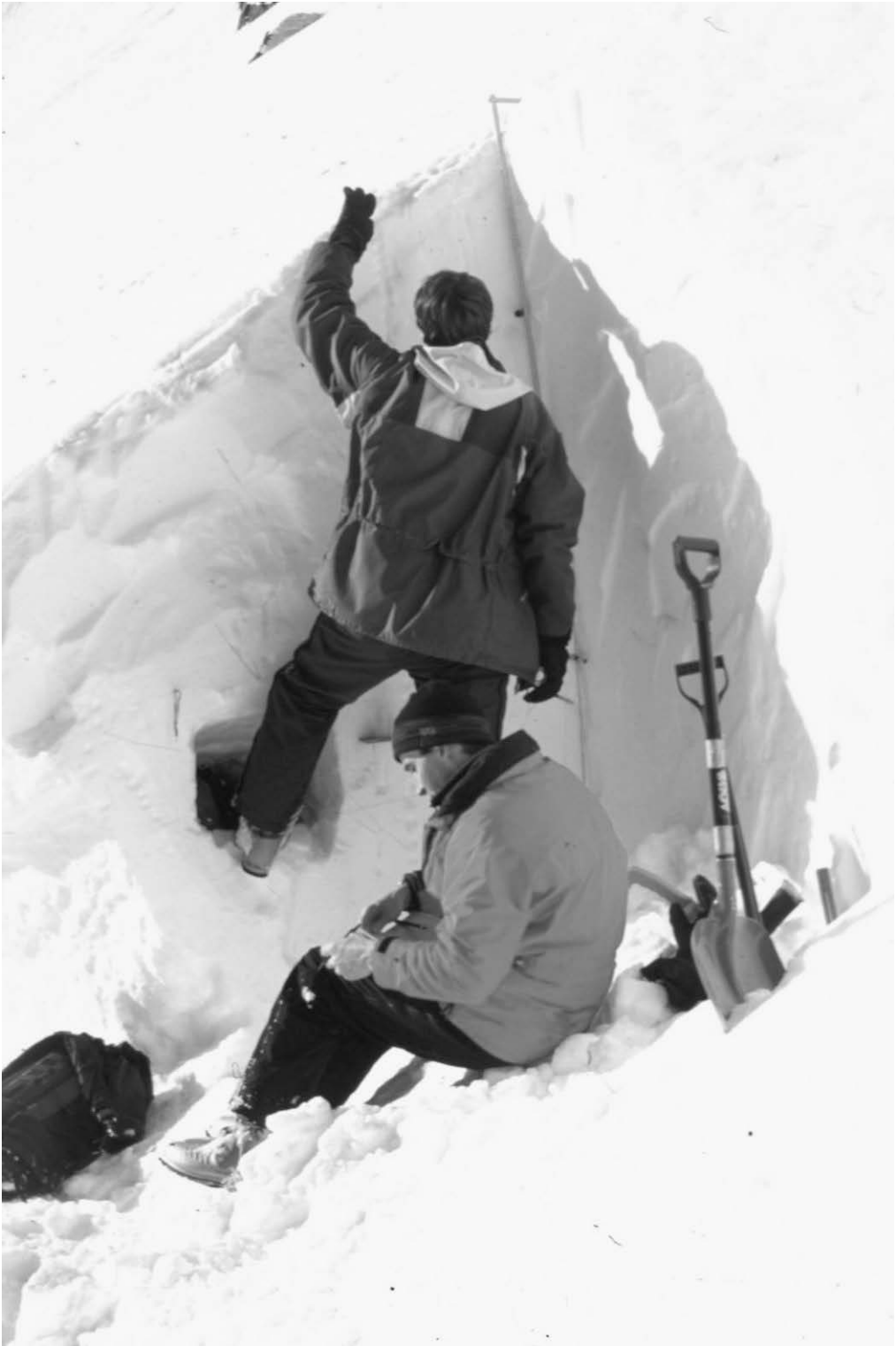
Figure 1.4. Avalanche investigators profile the snowpack at the crown fracture of a deep persistent slab avalanche after a fatal avalanche. Photo: Bruce Jamieson.
