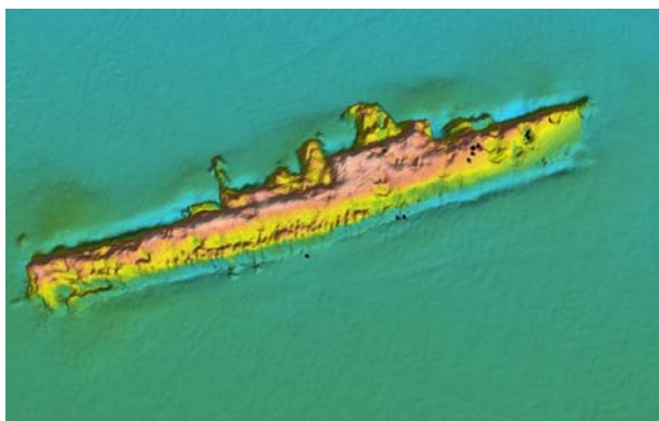
Figure 2. Side-scan sonar image of the HMCS Yukon showing the vessel laying on its port side. The bow of the vessel is oriented northward.
