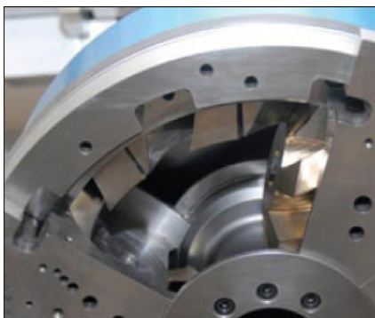
This Toroidal Intersecting Vane Machine, or TIVM, uses multiple chambers in a rotary torus configuration to generate high power density at slow speeds.
