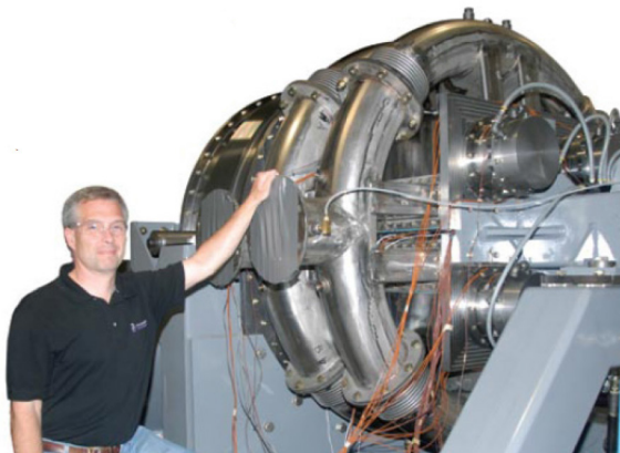
Concepts NREC designed, built, and programmed this rig used to test Mechanology's patent-pending Dragonfly compressor, a 500 hp positive-displacement oscillating vane machine.
