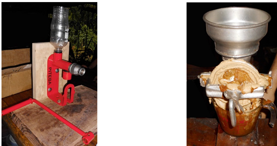
Figure 6. Press and hand mill, ready to press oil and prepare sacha inchi butter at household scale.
