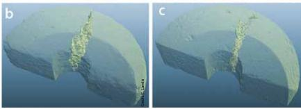
Figure 5. Analysis of reproduction of Trajan's Markets mortar. a) P. Brune performing a fracture testing experiment. X-ray tomography results for fractures at (b) 28 days or (c) 180 days of hydration.
