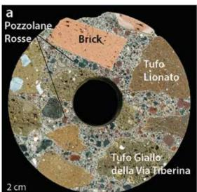
Figure 2. Drill cores of Roman concrete from a) Trajan's Markets in Rome and b) Trajan's Port (110–112 CE).<sup>2,3</sup>
