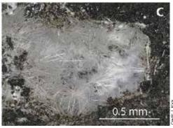
Figure 7. a,b) Surtsey volcano in Iceland is the location of the 2017 International Continental Drilling Program SUSTAIN project. c) Scanning electron microscope-secondary electron image of Al-tobermorite from SE-03 core at 124°C and a 147-m inclined depth.
