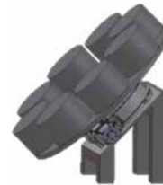
Moment load due to offset or inclined installation
