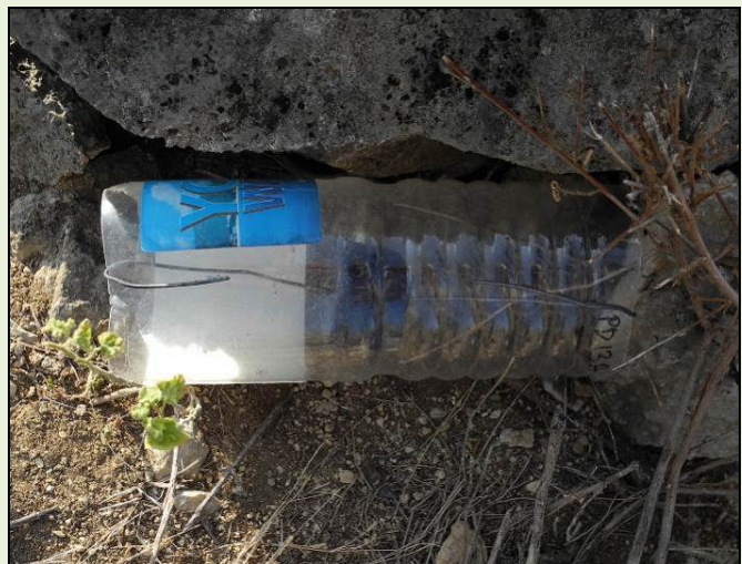
Figure 32. Example of goat-resistant bottle bait station for the ground-based phase of the black rat eradication (J. Daltry, FFI). Wire holds bait in place. Note entrance slightly raised off the ground to deter insects and crabs.
