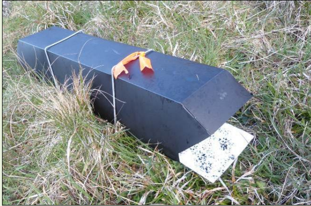
Figure 7. Example of a tracking tunnel in place (showing rat prints on card). (E.A. Bell, WMIL)
