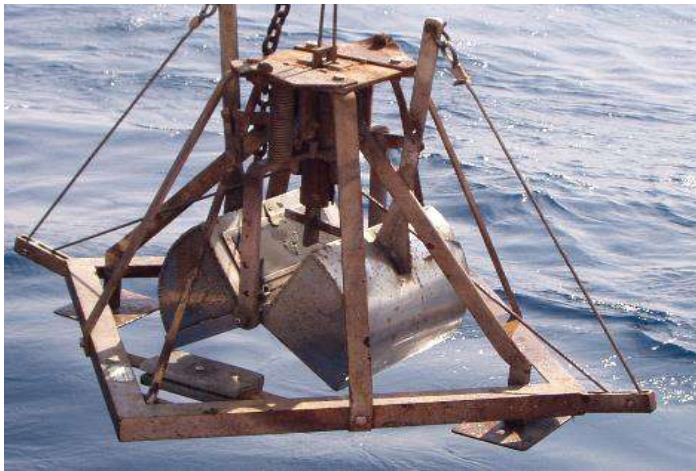
Fig.2. Smith-McIntyre grab, useful for collection of sediment samples for benthos (Photo courtesy: CMLRE)
