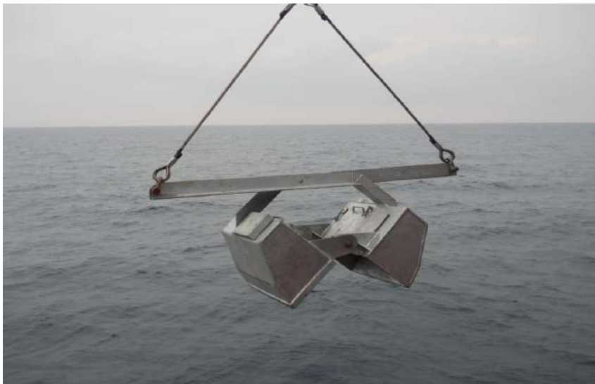
Van Veen Grab - for Seabed sediment sampling.
