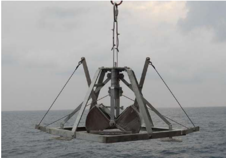
Smith Mc-Intyre Grab. – for Seabed sediment sampling.
