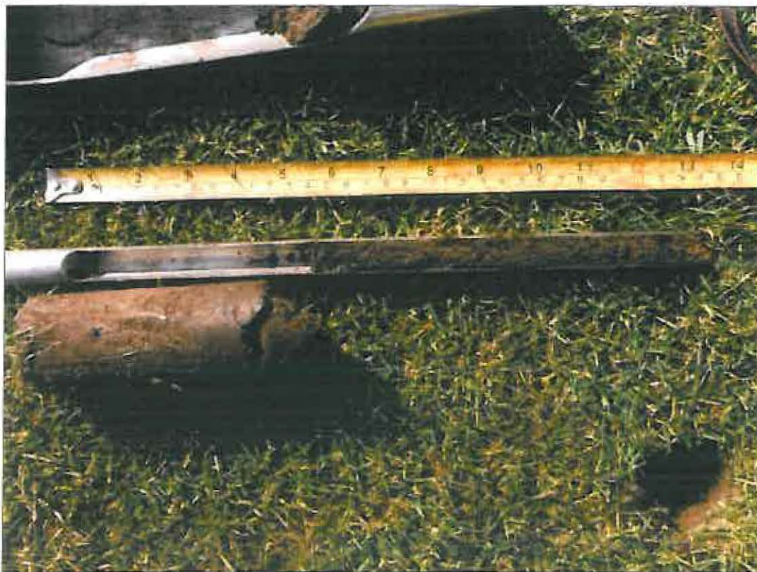
Soil auger samples showing the depth of the clay loam profile. Compaction was identified at 60-100mm depth.
