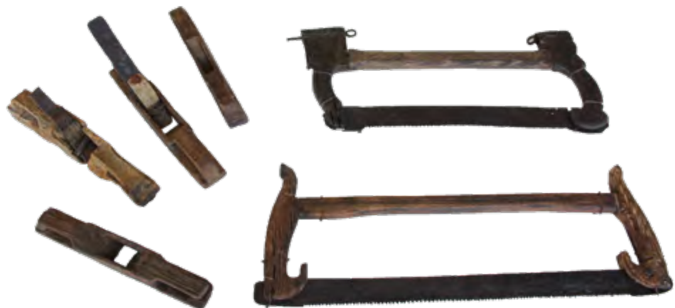
Figure 20.3 Four block planes and two bow saws from a carpenter's tool chest, found in the shipwreck De Meern I (photo: BIAX Consult).
