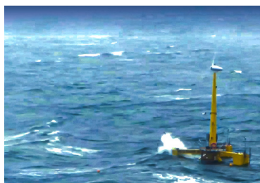
VoltturnUS 1:8 scaled 500-year storm conditions, 2013
