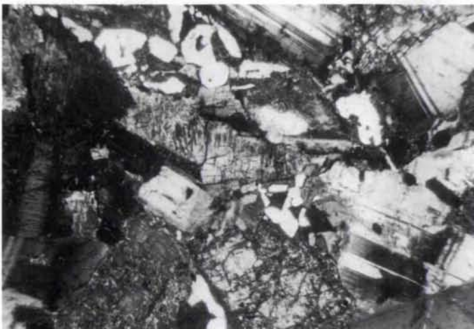
Figure 16. Intergranular texture in a coarse-grained zone. Textured gray mineral at center and bottom is partially altered pyroxene. Note micrographic intergrowths. Sample M11571; width of view 3.7 mm, crossed polars.
