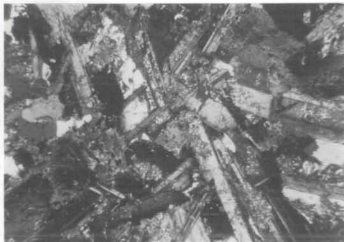
Figure 12. Cluster of plagioclase crystals between ophitic augite. Note that sericitization of plagioclase is more intense in the cluster. Sample M11535; width of view 3.7 mm, crossed polars.
