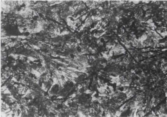
Figure 7. Photomicrograph of typical chilled margin. Note acicular Fe-Ti oxides and fan-shaped cluster of amphibole crystals. Sample M11556; width of view 0.9 mm, uncrossed polars.
