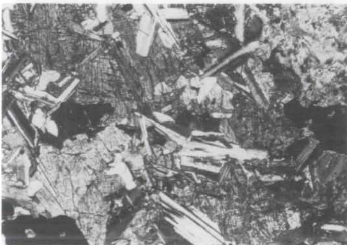
Figure 11. Ophitic augite. This composite ophite is made up partly of grains having slightly different optical orientations (e.g., the top part of photograph), and partly of grains having distinctly different orientations (compare top and bottom of photograph). Sample M11529; width of view 3.7 mm, crossed polars.
