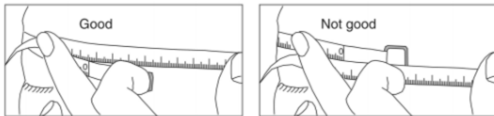
Figure 4. How to measure with a tape measure (Image from Kouchi, 2020).
