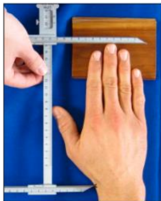
Figure 3. A caliper capturing the Hand Length measurement (Image from Gordon, Blackwell, Bradtmiller, et al., 2012).
