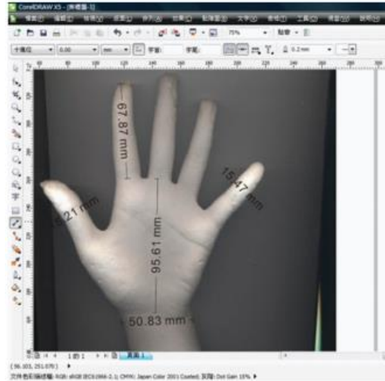
Figure 7. Hand dimension measurement extraction on a 2D image using CorelDRAW software (Images from Yu, Yick, Ng, & Yip, 2013).
