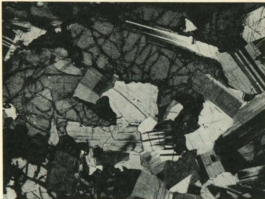
FIGURE 3.—Poikilitic olivine molded around plagioclase laths. This form of olivine is unusual, and indicates crystallization from the interprecipitate liquid. Sample M3716-3. 7\frac{1}{2}X , crossed nicols.
