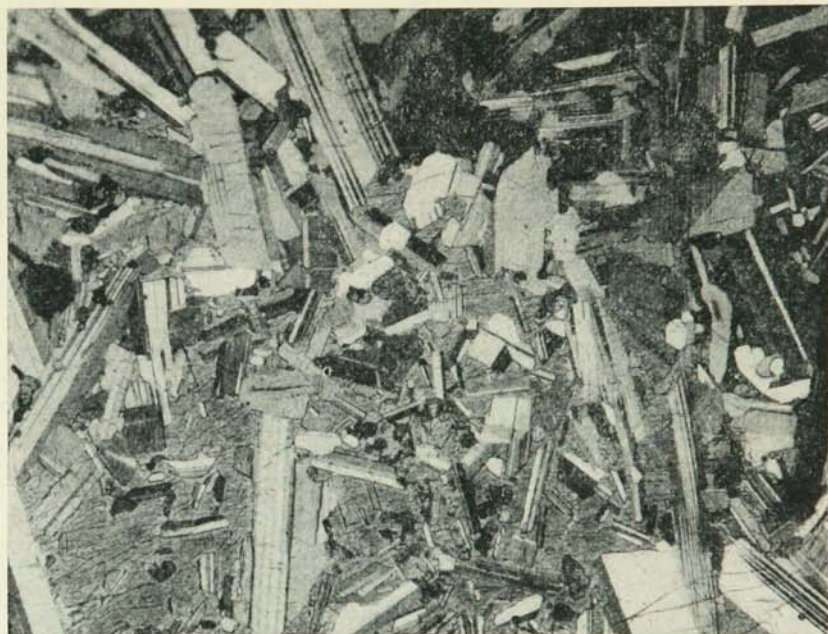
FIGURE 7.—Poikilitic augite enclosing rounded grains of olivine and small plagioclase crystals. The size difference between the plagioclase crystals enclosed in the augite and the crystals outside the augite indicates that the augite partly formed as a precipitate crystal, and by surrounding the plagioclase laths cut them off from additions by the interprecipitate liquid. Sample P55G. 7\frac{1}{2}X , crossed nicols.
