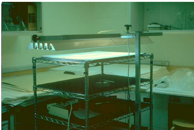
Fig. 6. Larger diazo test samples under light bank
