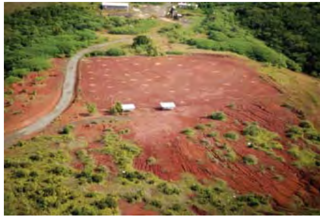
Figure 19.23 This baseball field, in Melekeok State in central Babeldaob, shows the problems faced when the laterite soils of Babeldaob are disturbed through land clearing and grading. The exposed soil is rapidly turned into erosion channels leading to local streams, which in turn feed into the Ngerdok (Shimizu) River. It is difficult to establish new ground cover on such soils, once disturbed. While several kilometers from the mouth of this river, the soil eroded into this watershed will accumulate along the river bed, degrading it as habitat for terrestrial organisms, and eventually affect the entire course of the river and the lagoon beyond.
