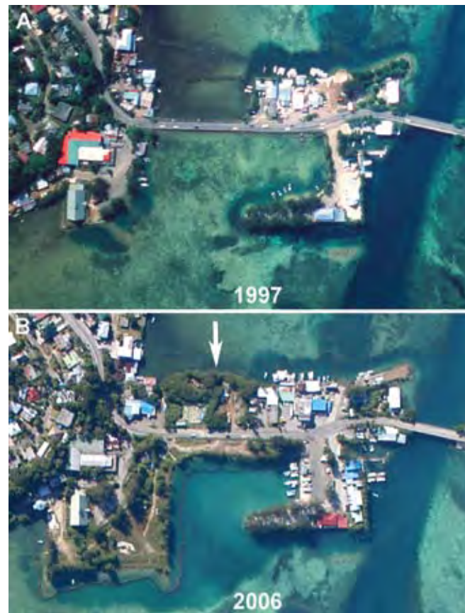
Figure 19.27 The urge and incentive to turn roadside running along the water into valuable and useful waterfront property is amply illustrated in this comparison of the causeway east of the Minato Bashi Bridge in Koror. The areas along the new land were dredged (to largely provide the fill for the land) allowing movement and mooring of boats in these areas. The area of the causeway on its upper side (indicated by the white arrow) was filled using red soil trucked in from elsewhere. The reddish color of the area is apparent and it still has the shallow flats along its shore since the area was not dredged for fill.
