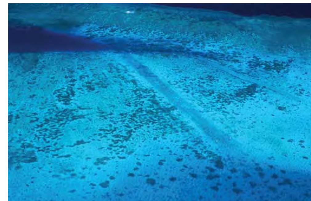
Figure 4.4 A new channel (center) through the western barrier reef at Kayangel Atoll was dug in 2003, replacing an older, shallower channel seen on the right side. While not particularly deep, the new channel allows access for small boats to the lagoon at all times. The reef in this area has coral patches (dark areas) on a white sand bottom, dropping to the deep ocean (dark blue at top) outside the atoll.
