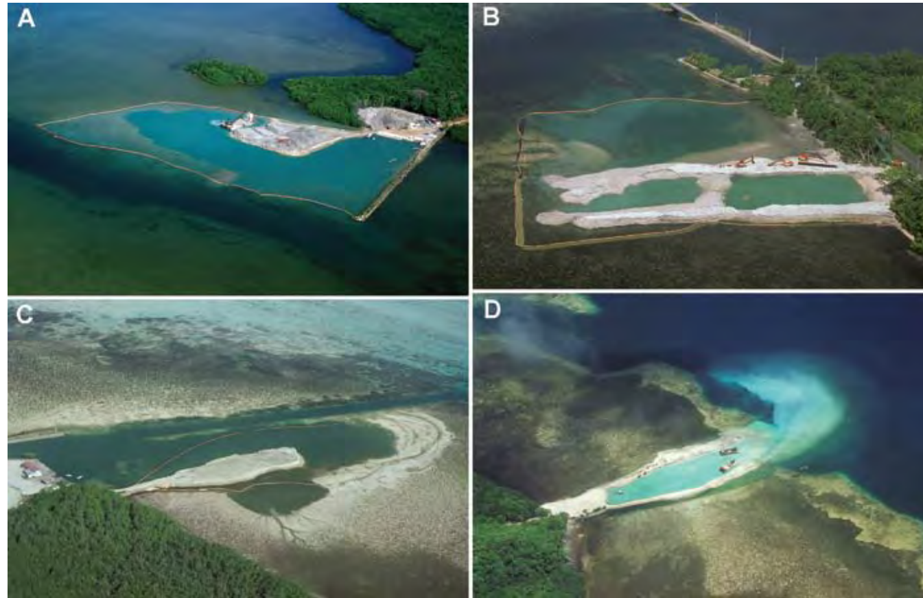
Figure 14.6 Coastal dredging of near-shore shallow flats was conducted for coral fill in many states on Babeldaob during construction for the Palau Compact Road. These dredge sites also now serve as small boat harbors; an extra benefit from the dredging. (A) Imul Village in Aimeliik State. (B) Ngijwal State. (C) Melekeok State. (D) Taprengesang in Ngchesar State. The silt curtain was not very effective on the day this photo was taken.
