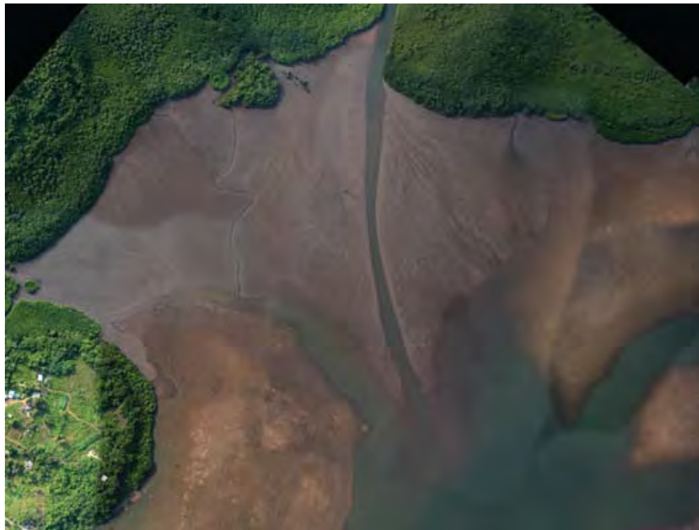
Figure 16.26 The mouth of the Ngerikiil River, at low tide, where it empties into Airai Bay. A large mud delta has been built out into the bay by soil washed down the river; the soil comes from erosion due to poor watershed-management practices upstream. The watershed includes a large number of farms. It was also the scene of Compact Road construction and major earthmoving for the extension of the Palau Airport runway. Much of the upper bay has a thick coating of sediment on the bottom. Living coral reefs have been eliminated in this area.
