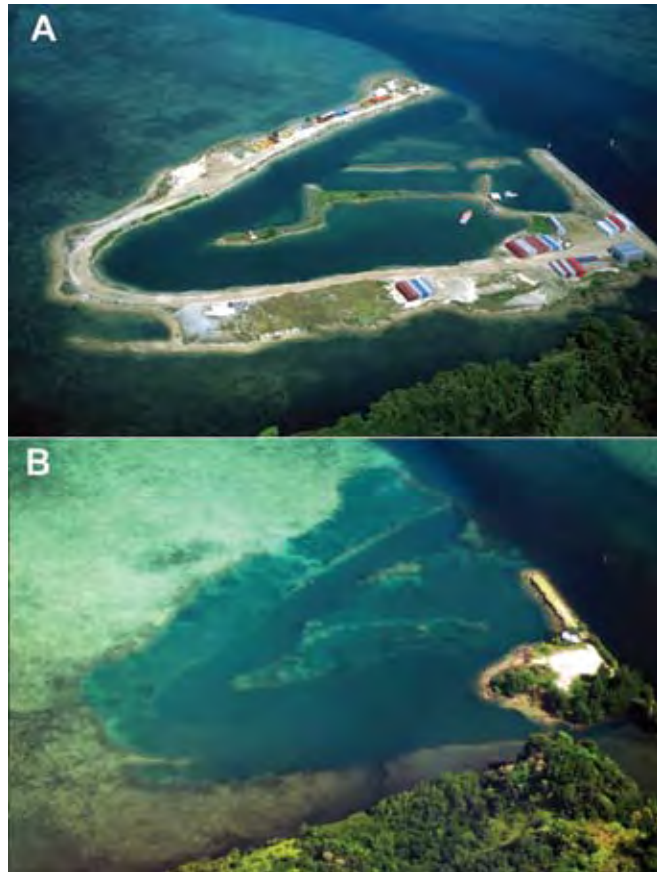
Figure 15.2 There has been much dredging for fill materials in Palau, mostly for road construction and harbor development. (A) During construction of the Urung causeway in Ngaraard State for the Palau Compact Road in 2003, a temporary port was developed by dredging up berms and digging a basin on the lagoon side of Babeldaob. By the end of the road project, virtually all of this berm material had been removed, having been used as fill for the Compact Road or for projects elsewhere. (B) In this view of the same area in 2009, the former harbor area has had nearly all the former berms removed by dredging them down as far as an excavator could reach. There are no apparent effects on the nearby shallow flats around the island from this dredging activity, but there has not been any on-site monitoring of any of these dredging projects to assess impacts in detail.
