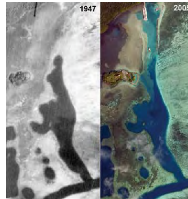
Figure 3.44 The northern leg of the Toachel Ngedbaet is a natural channel which has been dredged over the years so that it now extends to the shore. The area now contains a fishing dock and a depot for fill materials dredged up from the reef.
