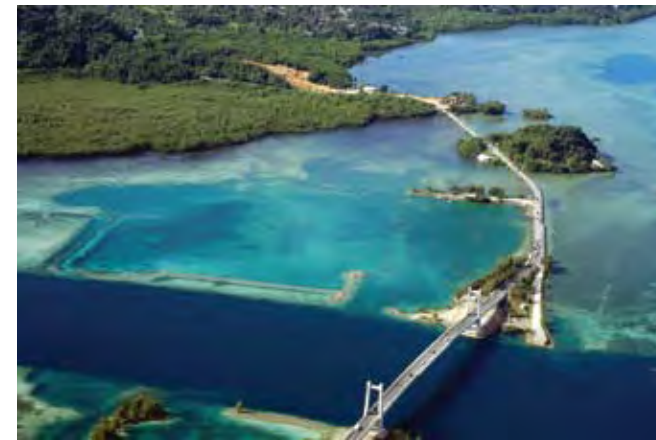
Figure 15.6 This large area on the Koror side of the KB bridge was dredged for fill by mechanical excavators; the dredging took place over many years. This oblique aerial photo indicates that some re-growth of benthic communities (dark areas within dredged sites) has occurred. However, this re-growth has not been well documented. In general, there is little followup to see how areas do or do not recover from human activities.
