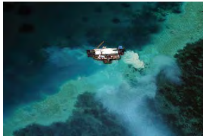
Figure 15.4 Submarine coral-sand mining has been going on for many years on the lagoon side of Lighthouse Reef. A barge-based suction dredge (at the rear of the barge) dumps uplifted sand onto the surface of the barge, where the water flows off the sides while the sand remains in piles on the barge. Once the barge is full of sand, the tugboat tows the barge and crane back to shore, where the sand is offloaded onshore by the crane. The water flowing out of the sand dumped on deck carries a high load of fine sediment, but much of the sediment dredged remains on the barge surface and becomes part of the harvest. This sand is used for construction and for building artificial beaches around Koror. While seemingly damaging, the operation appears to have had little, if any, direct negative effect on the Lighthouse Reef area.
