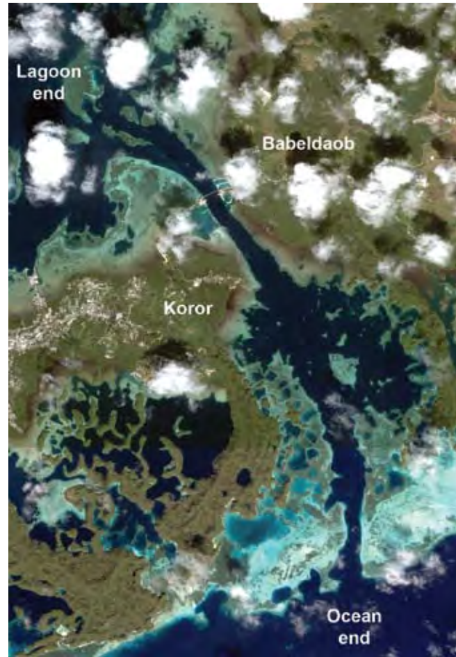
Figure 3.36 This satellite image shows the Koror-Babeldaob (KB) Channel in its entirety. The total channel is about 8 km in length. Its narrowest portion, at the bridge, is only about 250–300 m wide. The central area, between the bridge and the ocean end of the channel, has a complicated bathymetry, with deep sides and many shallow reefs. Currents through the channel are strong and are reported to range up to 7 knots in speed. It is likely this channel was an ancient river bed during the last glacial low water. Satellite image courtesy Palau Automated Land and Resources Information System (PALARIS).
