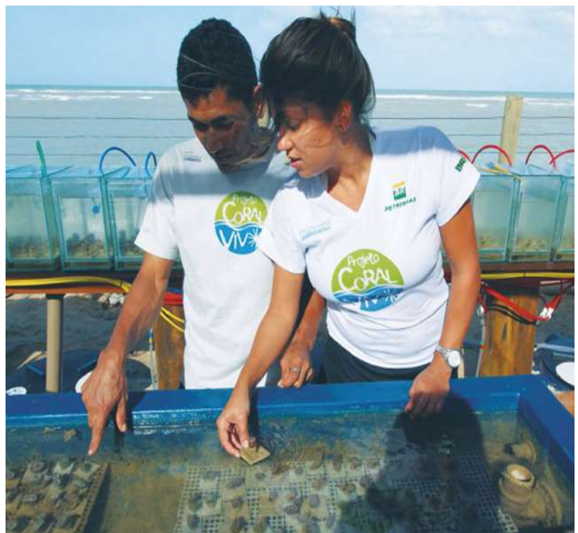
Figure 2. Experiment of seawater acidification, increasing temperature and micronutrient (copper) enrichment conducted in the marine mesocosm facility of the Coral Vivo Project, Arraial d'Ajuda (Porto Seguro, Bahia, northeastern Brazil).
