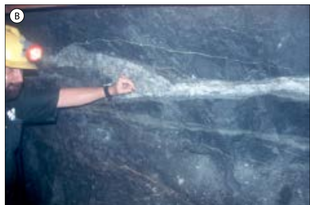
Figure 3.47 Development of ore hosting flatmakes at the Emperor gold mine, Fiji. A - Structure of the mine area with different colours to distinguish collapsed blocks within the wall rocks adjacent to the Tavua caldera and flatmakes shown in red. D - Flatmake in the mine workings.
