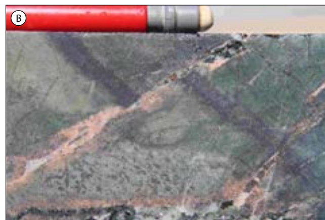
Figure 3.56 Cadia East wallrock porphyry. A - Sheeted A type quartz veins with auriferous pyrite and Mo and K-feldspar alteration selvages. B - Down-drop on veins-hosting fractures within the wall rock.
