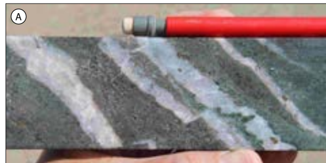
Figure 3.55 Sheeted quartz vein formation at the Goonumbla district, Eastern Australia. A - Sheeted quartz veins from the E26 porphyry in hand specimen. B - Sheeted quartz veins showing bornite mineralisation from E48 porphyry. C - Geological setting of the E 26 and E48 porphyry systems, from Owens et al., in press; and Corbett and Leach, unpubl. report, 1995. D - Legend
