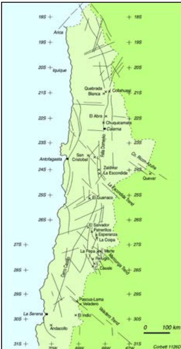
Figure 3.2 Structures in Northern Chile including the Falla Oeste-Domeyko Fault system which localises many porphyry systems and epithermal deposits, locally at the intersections with conjugate fractures. See figure 3.5A for location.
