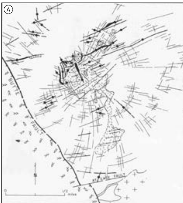
Figure 3.51 Different quartz vein configurations formed in varying structural settings. The sheeted veins in the transpressional setting may rise above the porphyry environment to form wallrock porphyry deposits.
