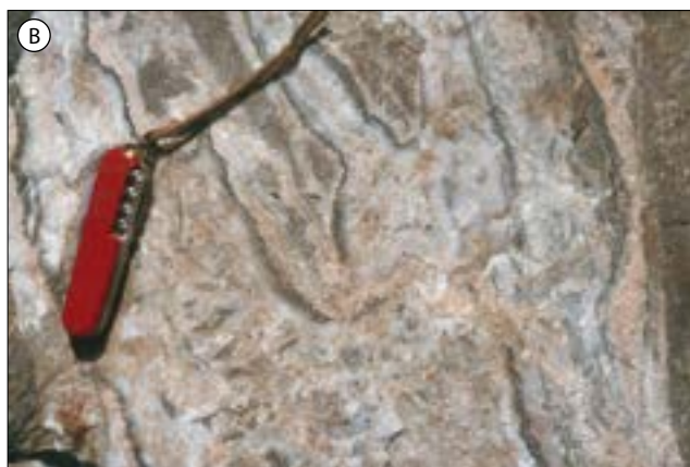
Figure 3.22 Golden plateau, Link structure, Cracow goldfield, SE Queensland. A - Plan illustrates the Golden Plateau link structure formed by interpreted sinistral strike-slip movement on the two controlling structures which host numerous small gold showings (from Brooks, 1971). B - Banded quartz adularia vein/breccia from Golden Plateau. C - View showing Precipice Sandstone cover.
