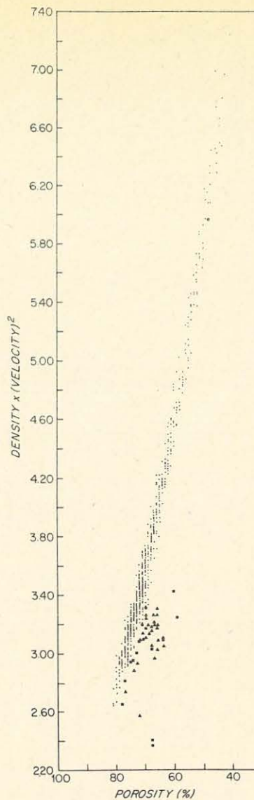
FIG. 15. Plot of density \times ( in-situ velocity) 2 versus porosity for sediments from Hatteras and Nares Abyssal Plain cores. Bold symbols show samples with grain densities \leq 2.50 g/cm 3 : triangles—from cores RC19-27, 28, and 29; squares—from cores RC19-20, 32, 33, 36, 37.
