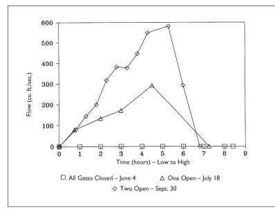
Figure 5. The flood tide on June 4,1992 with all gates closed, July 18,1992 with one gate open, and September 30,1992 with two gates open, West River, New Haven, Connecticut.
