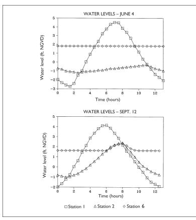
Figure 4. Water levels at station 1 (immediately downstream from the tide gates), station 2 (30 m upstream from the tide gates), and station 6 (at the Whalley Avenue bridge) (see Figures 1 and 2), on June 4, 1992 with all gates closed and September 12, 1992 with two gates open, West River, New Haven, Connecticut.
