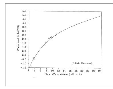
Figure 8. A function [Y = 2.65 (In X) - 3.8] relating water surface elevation (Y, ft) to water storage volume (X,  $10^6$  ft<sup>3</sup>) developed from topographic data for the West River Marsh, New Haven, Connecticut. The triangles superimposed on the function show the water surface elevation at high tide versus total volume of inflow calculated by numerical integration from tidal discharge data collected for six events during July through September, 1992.
