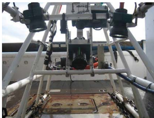
Figure 10. T.V. sledge and camera equipment used for DDV tows
