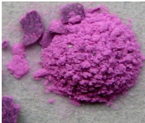
Fig. 1.14: image of the \text{CaCoSi}_2\text{O}_6 pyroxene synthesized at P = 3\text{GPa} and T = 1200^\circ\text{C}
