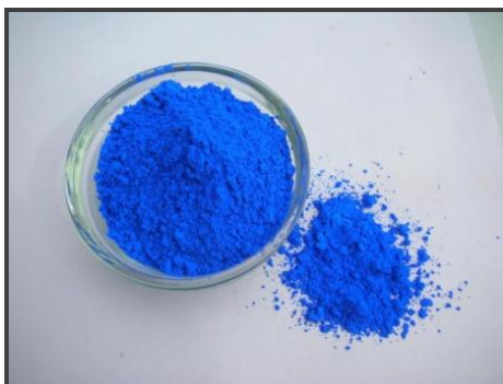
Fig. 1.3: images of the powder of Co-aluminate spinel ( \text{CoAl}_2\text{O}_4 ) known as "blue cobalt" (from www.cemcraft.com )
