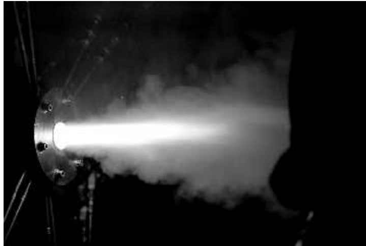
Gelled propellant engine test: 55-wt % RP-1/Al.
