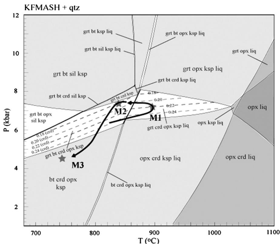
**Fig. 4.** P–T pseudosection in the KFMASH model system for pelitic granulite (sample 92378-1) with M1 peak assemblage grt–crd–opx–ksp, shows the crossing of the univariant reaction  $\text{grt} + \text{bt} = \text{crd} + \text{opx} + \text{ksp} + \text{liq}$  through a prograde heating.
