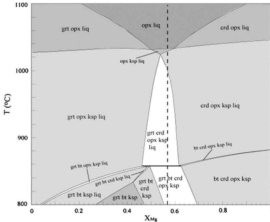
Fig. 5.  $T$ - $X_{Mg}$  pseudosection at 7.0 kbar in the KFMASH model system for sample 92378-1 indicates that its bulk composition is of an  $X_{Mg}$  value of 0.57 along the dashed line, and phase relations vary with changes in temperature.
