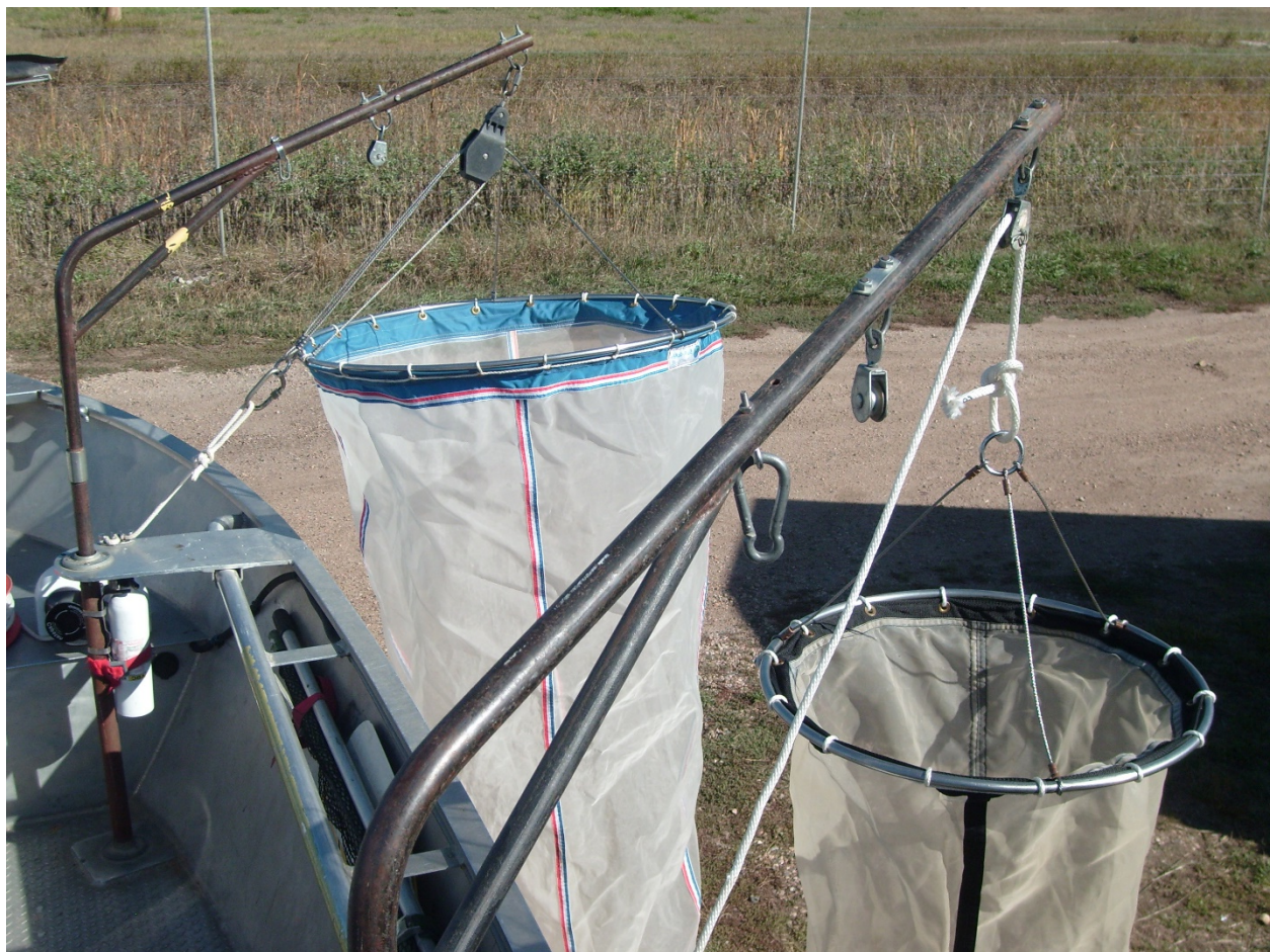
Meter and half-meter diameter plankton nets used for Mysis sampling during this study.
