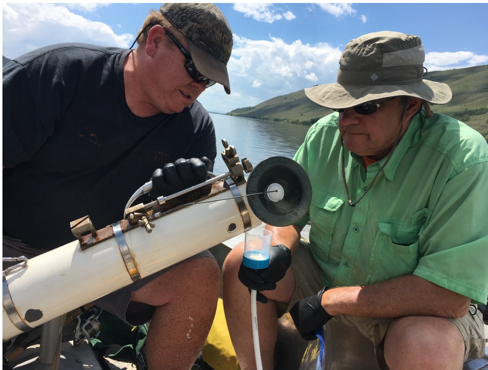
Bill Pate and Doug Silver collecting an environmental DNA (eDNA) water sample to detect Mysis (B. Johnson, Colorado State University).
