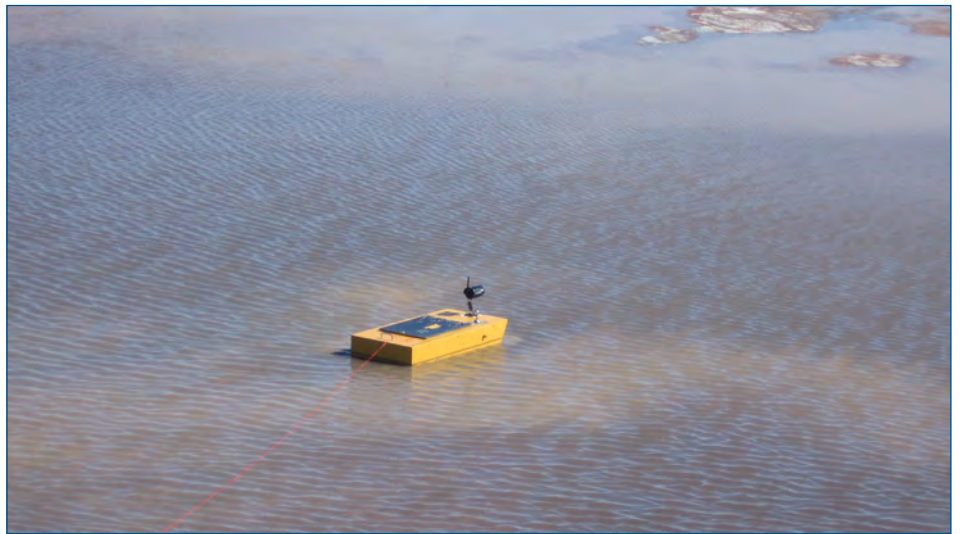
Plate 8. The radio controlled boat (RCB) on its way to collect a sample, January 2008
