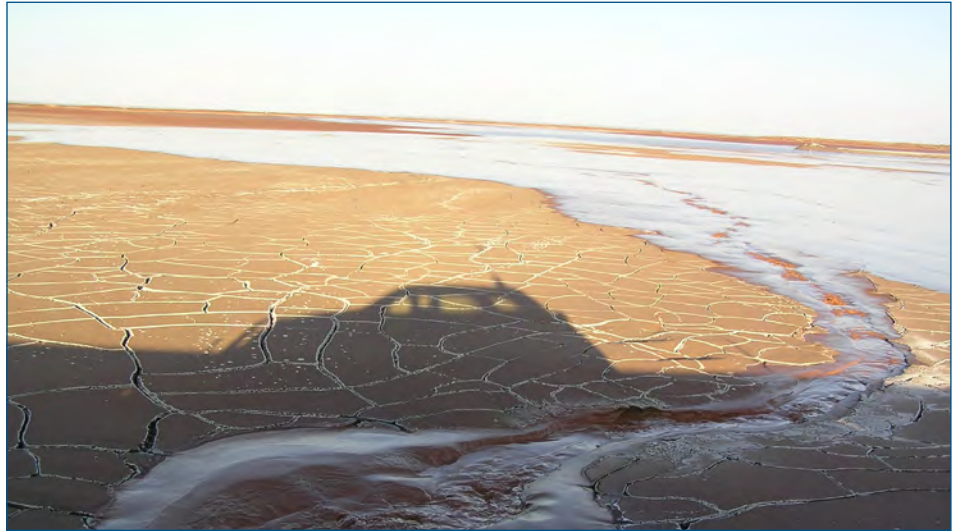
Plate 1. Tailings discharge showing spigot pool, channelled stream and sheet tailings flow, May 2010.
