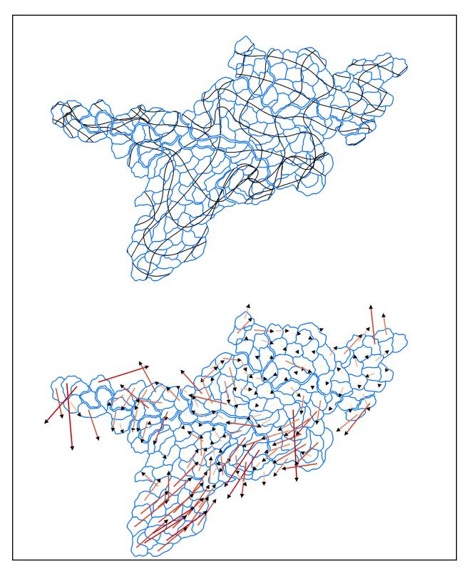
**Figure 6.** MapAnalyst generated 'distortion grid' (top) and directional displacement vectors (below) projected onto Loughinsholin townland boundaries as digitized from MPF 1/47.
