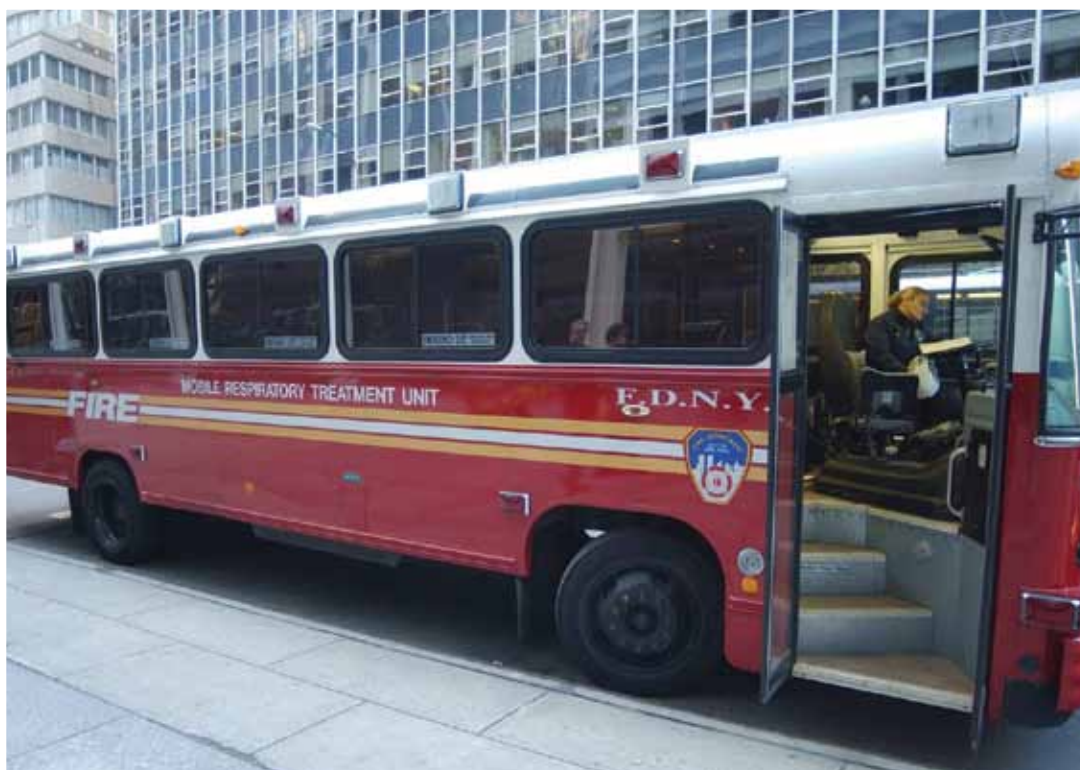
Shown above is a mobile respiratory treatment unit (MRTU), which has multiple oxygen outlets located through to provide oxygen to multiple patients simultaneously.
