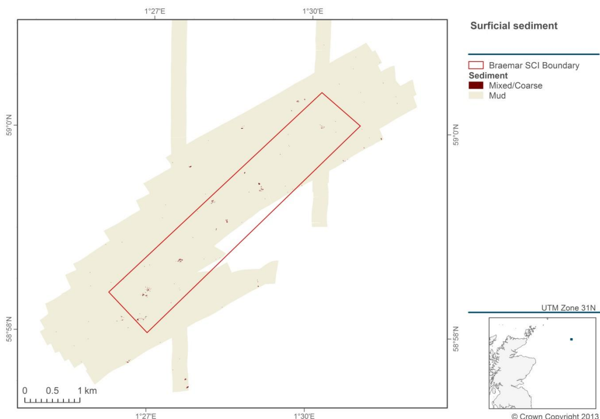
Figure 13. Sediment classification map of the Braemar Pockmarks SCI based on the combination of acoustic and groundtruthing data.
