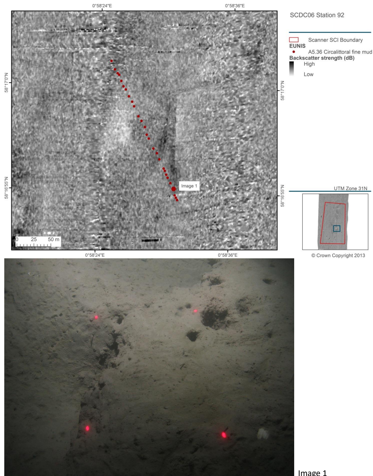
Figure 43. Close-up detail of Station 92 within the Scanner Pockmark SCI. Still image shows an abrupt change in seabed elevation at the scale of a few centimetres.
