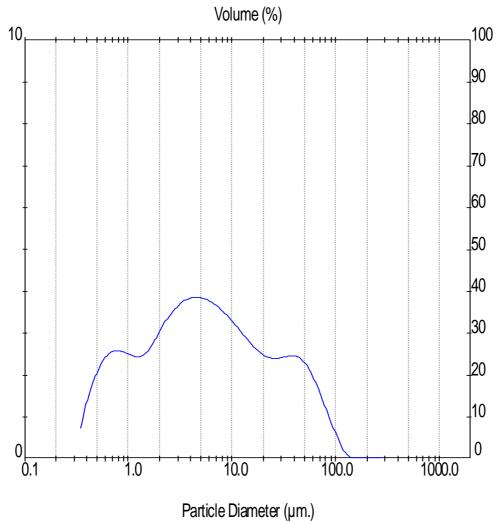
**Figure 64.** Laser diffraction test results for site 18.1, area 4
