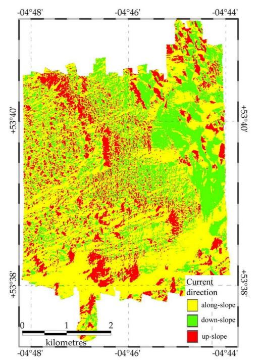
**Figure 25.** Aspect image of Area 3. Aspect is categorised according to dominant tidal current direction (azimuth 68°).
