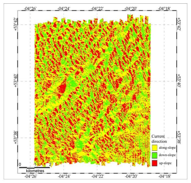
**Figure 16.** Aspect image of Area 1. Aspect is categorised according to dominant tidal current direction (azimuth 83°).
