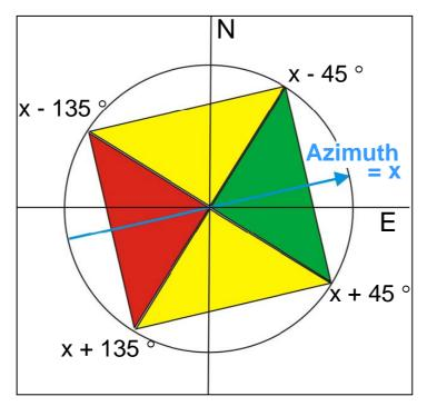
**Figure 8.** Classification of aspect values. Blue arrow: azimuth of the dominant tidal current direction.
