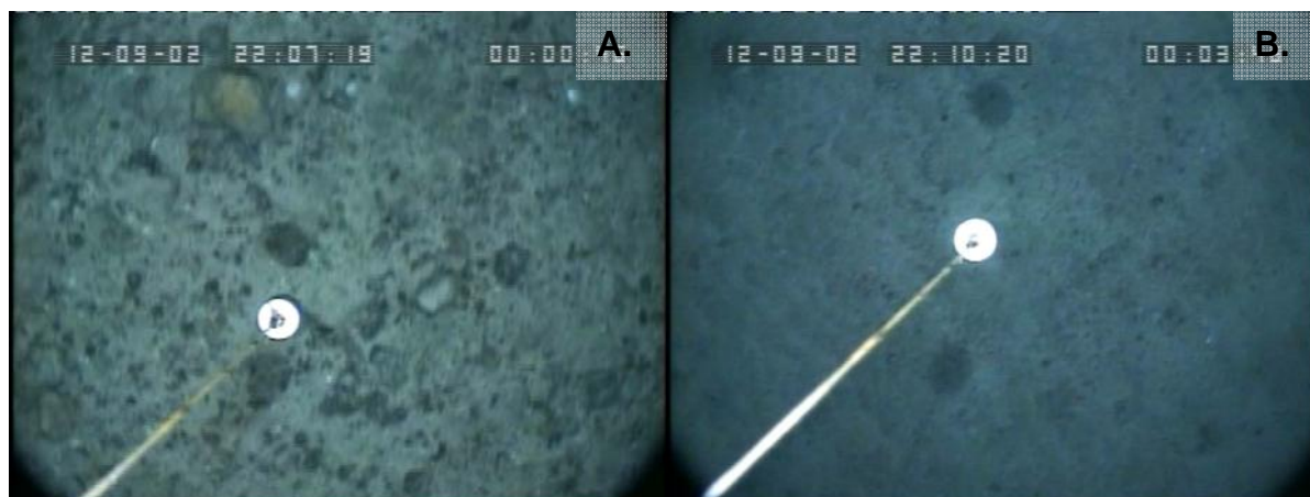
Figure 3.8 Video footage snapshots from station DW02008. A) Cobbles and boulders present on mixed sediment; B) Sand sediment.
