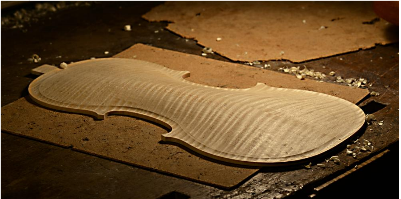
Fluting channel of the back
