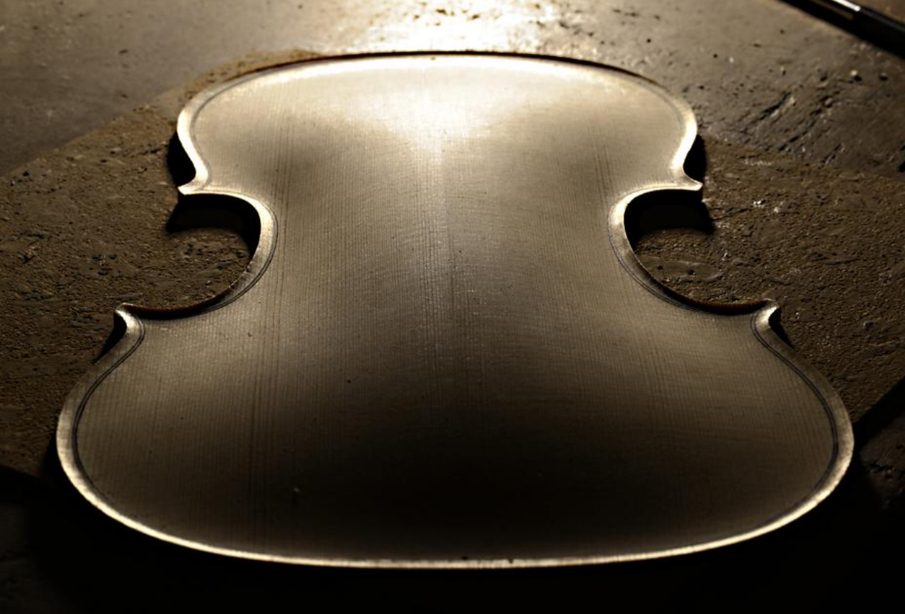
Finished top plate arching
