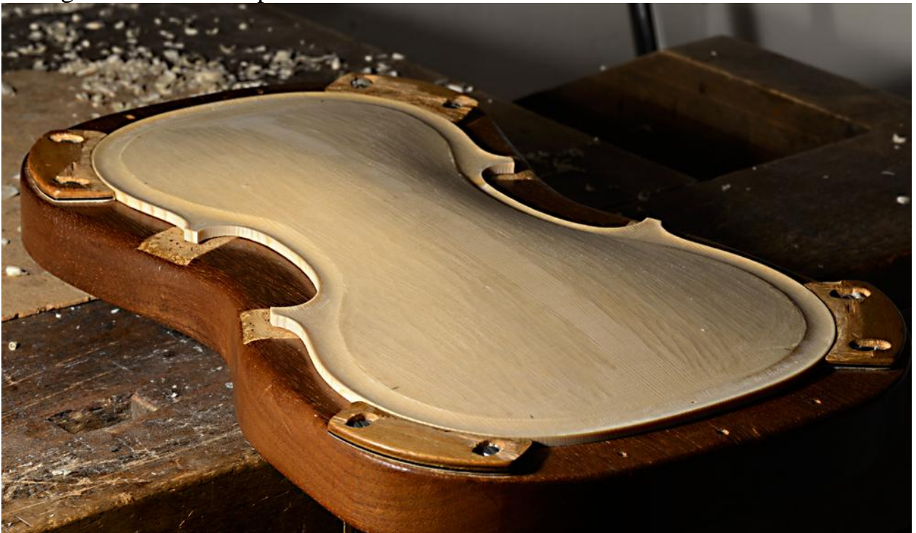
Fluting channel of the top
