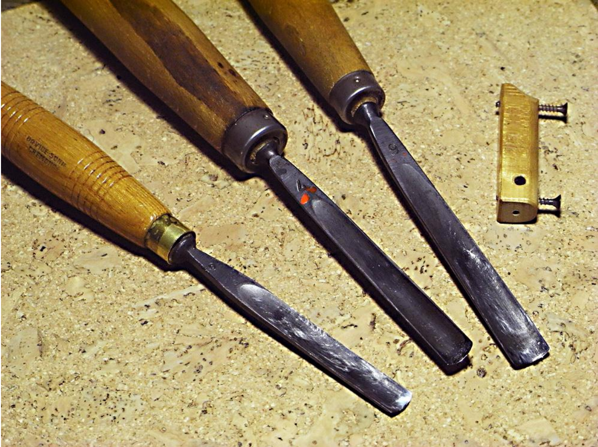
Gouges for the channel and marking gauge to mark the widths of the channel
