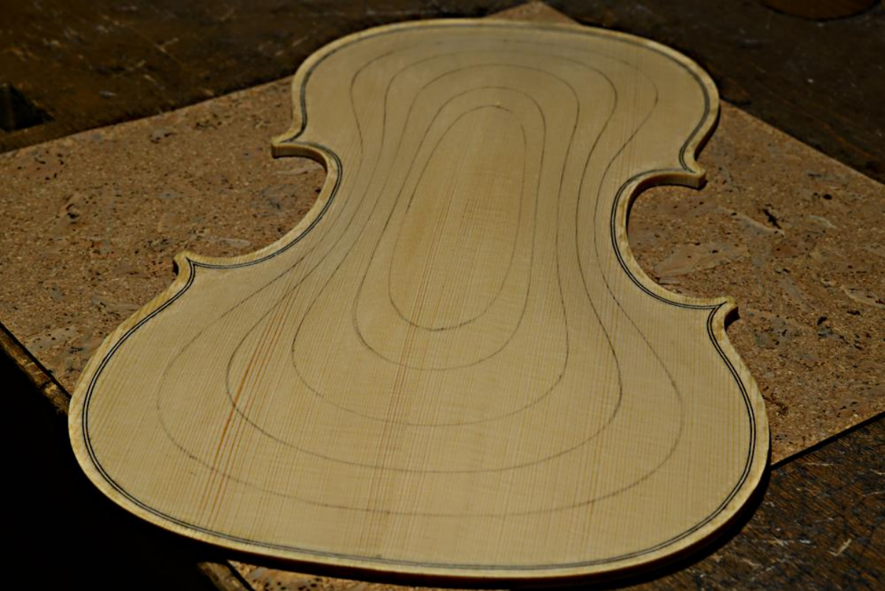
Top plate contour lines
