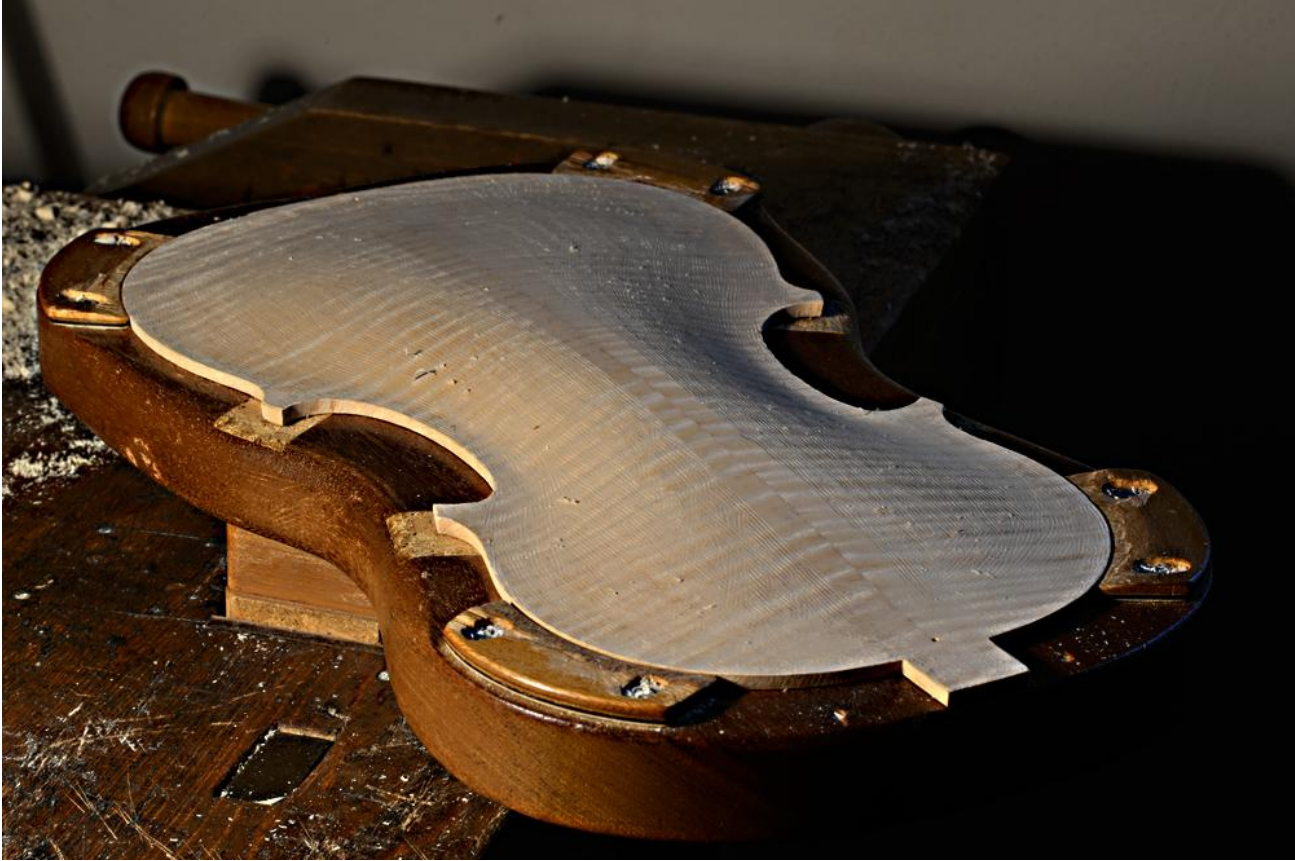
Back roughed with toothed blade fingerplane
