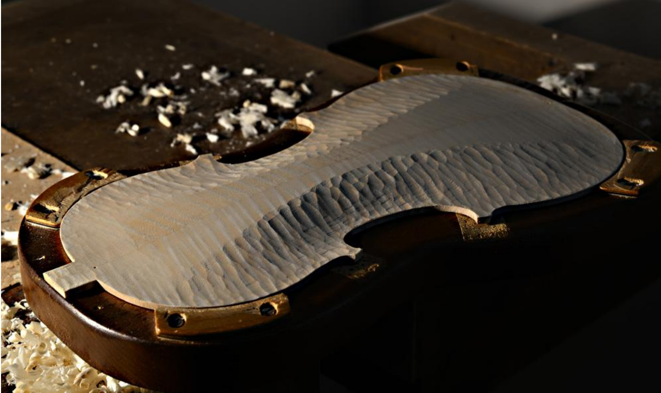
Back plate sixth finished with planes
