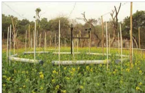
Free Air Carbon dioxide enrichment (FACE) facility built in JNU. Mustard (Brassica) plants are grown inside FACE Rings maintained at elevated CO 2 (550 ppm)
