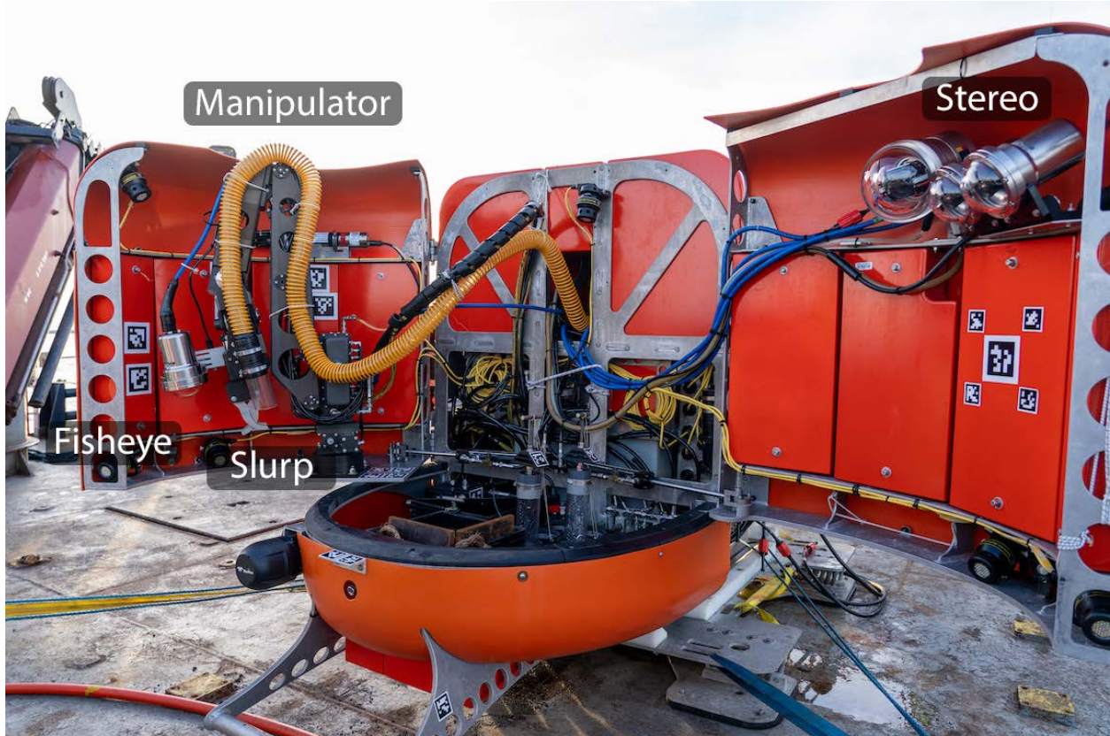
Figure 6.14: The NUI vehicle is outfitted with clam shell doors that can be closed to reduce drag when cruising and opened to perform manipulation tasks. The manipulator is mounted to the starboard door and the stereo cameras are mounted to the port door.
