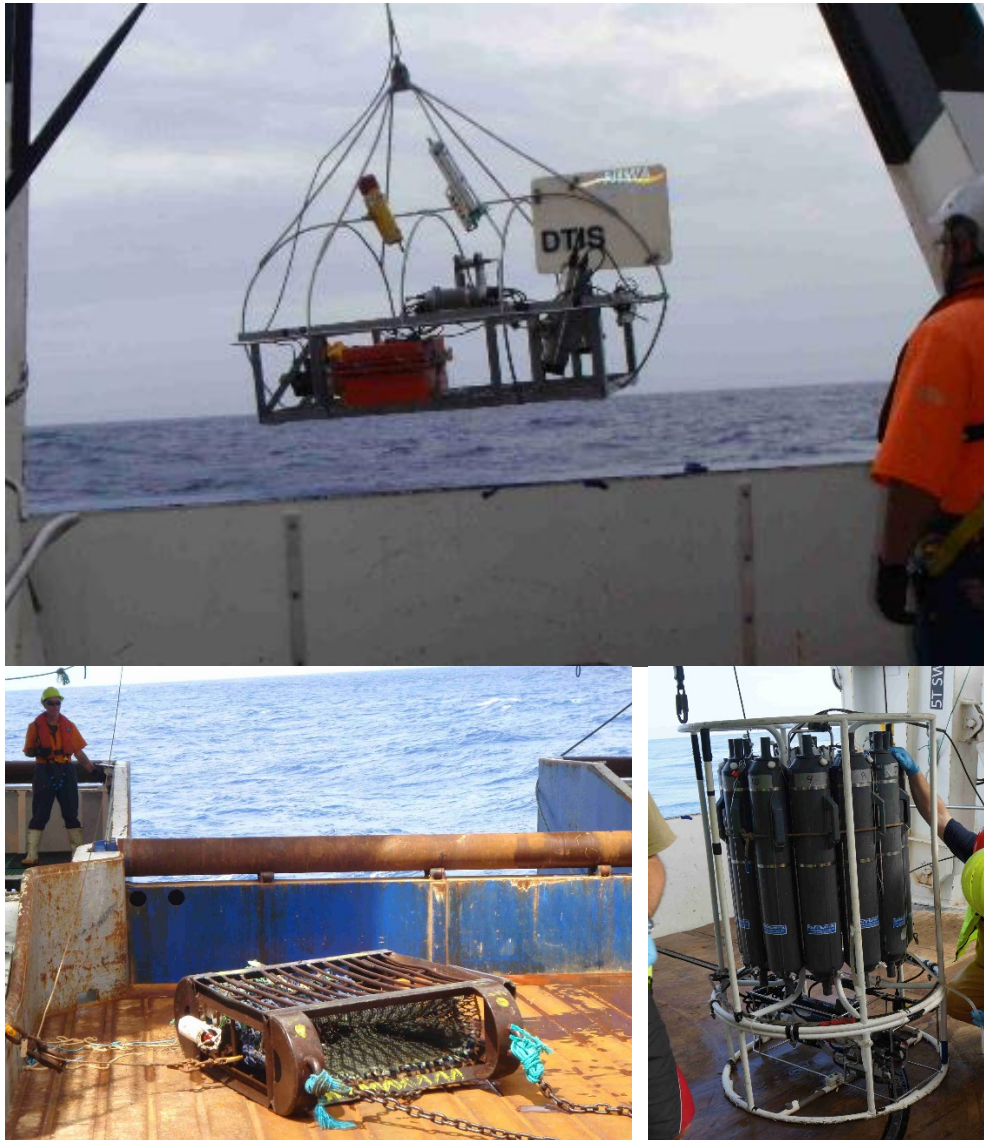
Figure 3: The sampling gear used for the survey: DTIS (top), the Seamount epibenthic sled (lower left), and 12 bottle CTD (lower right).
