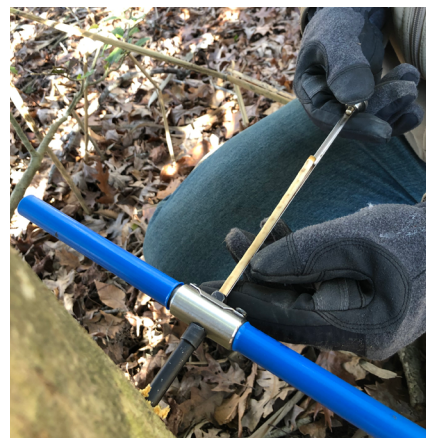
Figure 3. Coring an American holly with a Haglöf 5mm increment borer.
