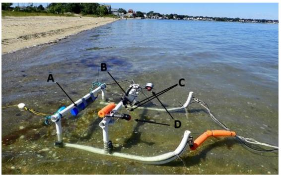
Figure 1. Photo depicting benthic sled configuration. A) Eureka Manta 2; B) SeaView Camera; C) Lasers; D) LED lights.
