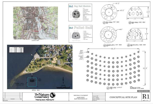
**Figure 11.** proposed reef layout showing the intended array of reef modules consisting of Pallet Balls and Bay Balls.
