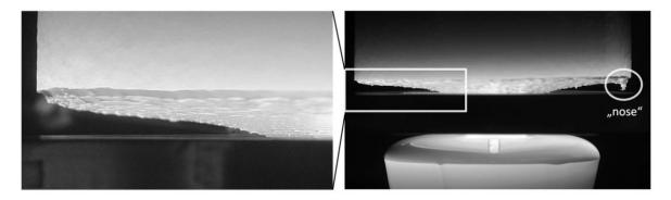
**Figure 5-4** The open melting front and formation of a large "nose" during the FZ process. The liquid silicon does not homogeneously cover the feed rod front. The formation of a nose is often observed at the rim of the feed rod.
