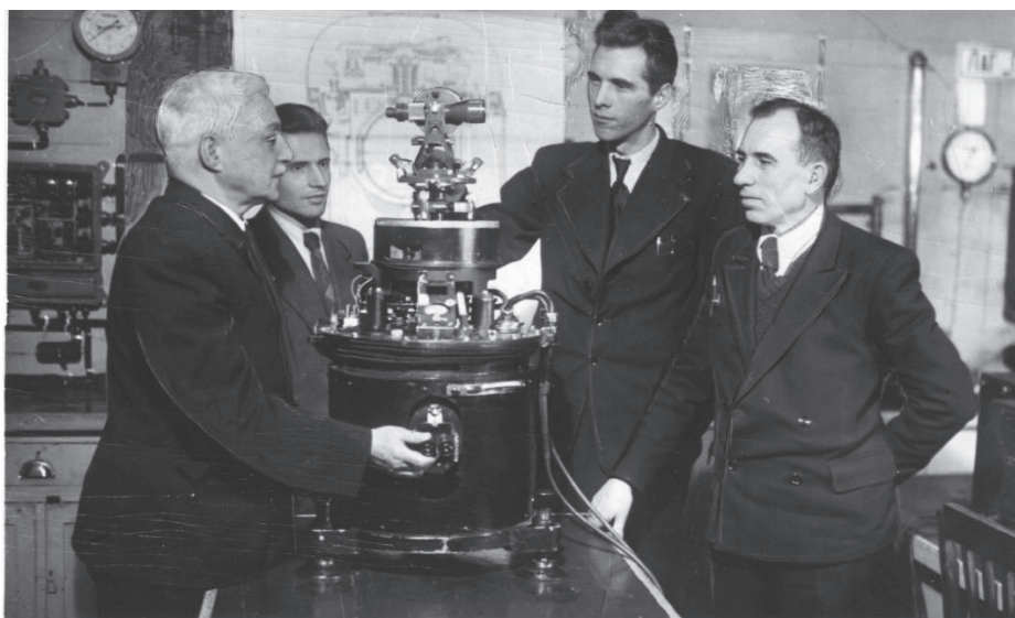
Fig. 1.1. Head of the Department of Navigation Instruments Professor K.S. Ukhov (first left) and staff of the department (from left to right): AA. Zeletenkevich, I.V. Ivanov and PA Il'in – testing the survey gyrocompass M-1. Photo of 1950 [https://museum.ifmo.ru/pages/128/140/]
