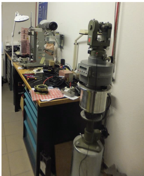
Fig. 1.9. Calibration of collimator with GYROMAT 2000
