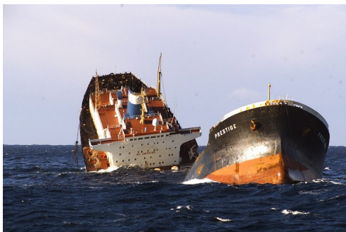
Fig. ii. Prestige's hull breakage just before sinking (Photo EFE).
