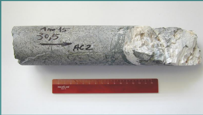
Drillcore from borehole AC2 (Cabeço de Vide Spa). Serpentinized dunite, showing the presence of serpentine (s) and brucite (b) along fractured zones.
